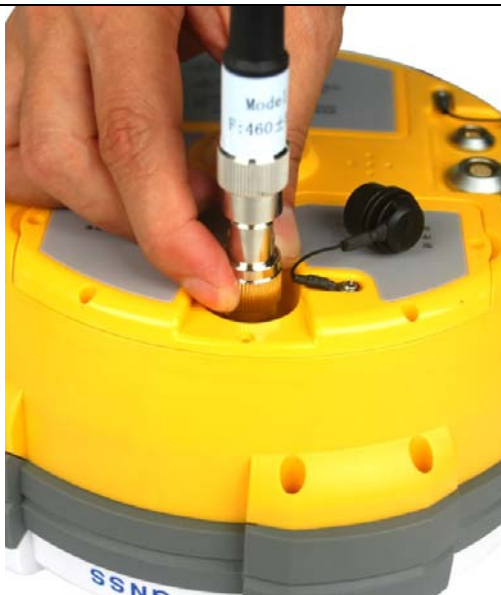
Figure 8-4 Differential Antenna installation
